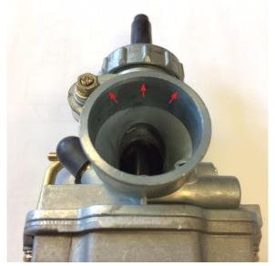
At the choke bore ID (sometimes referred to as the air horn) on the PZ22 and PZ26 a slight chamfer to remove any burrs left during facing of the inlet lip may be present. This is not new to the manufacturing of our carburetors but a recent concern and reason for this bulletin is that the finish appearance of this chamfer has changed.
