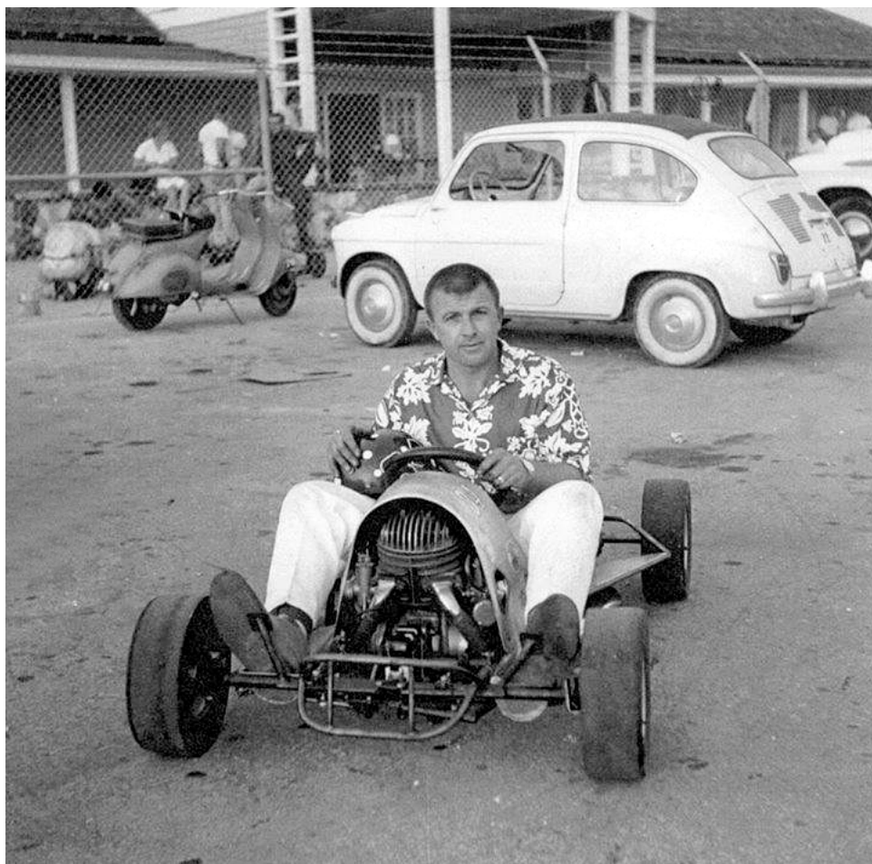
Duffy in his front engine experimental kart, powered by a 20 HP Puch built in 1960.
